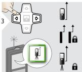
Distance is measured from the rear of the device (standard setting).
